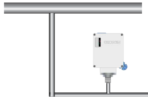
Installation under the pressure fitting
